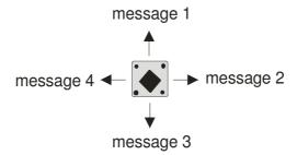
To start recording mode push the PLAY/REC joystick into one direction (depending which message you would like to record) and hold the stick in this position. After the beep you can start with recording and stop recording when you hear two short beeps. REC/PLAY procedure is indicating by REC/PLAY LED as well. REC/PLAY LED is flashing during recording or playing procedure.
